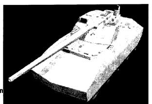
The FCS Anti-Tank variant is a 20-ton vehicle with a 2-man crew and a direct fire ETC weapon capable of beyond-line-of-sight fires with the Tank Extended Range Munition (TERM) round. The gun elevates up to 60 degrees to enable precision fires at elevated targets in urban environments with programmable levels of lethality.
