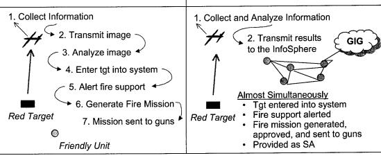
As an example of how current and future capabilities could differ, compare the operation of the current ABCS system with the potential of the future Tactical InfoSphere.
